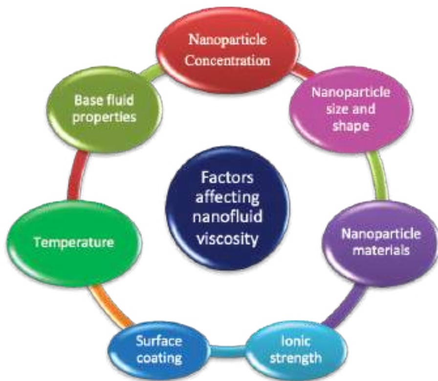
Figure 7. Factors affecting viscosity of nanofluid.
