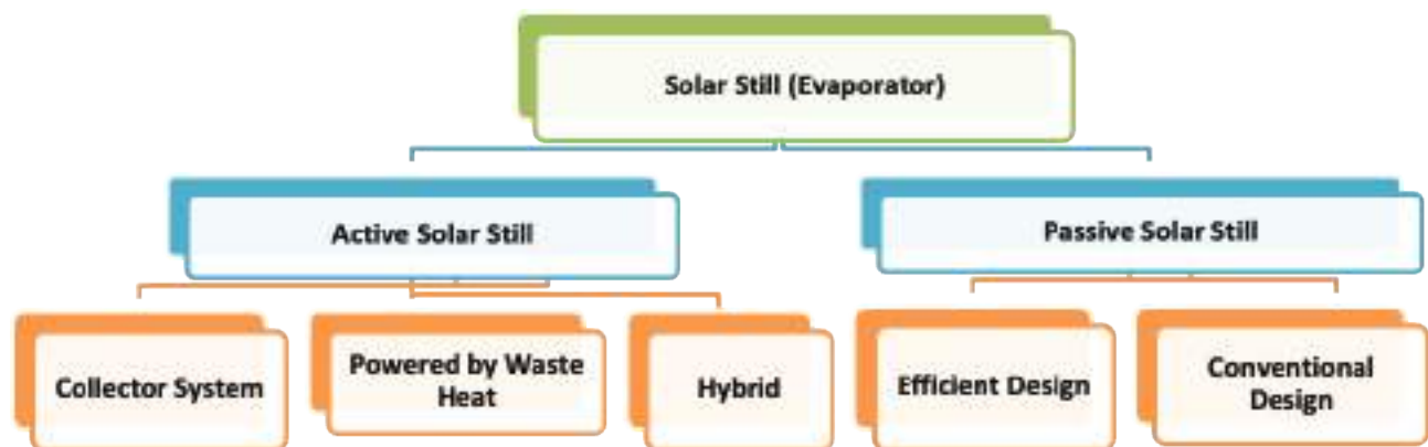
Figure 20. Classification of Solar Still (Evaporator).
