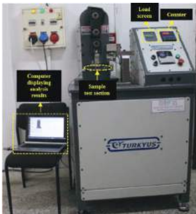
Figure 4. Schematic view of the flexural fatigue test system specially designed for this study and test machine image.
