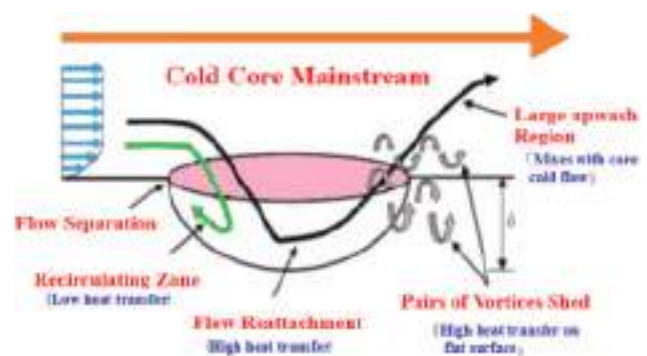
Figure 8. Plausible flow structure of dimple.
