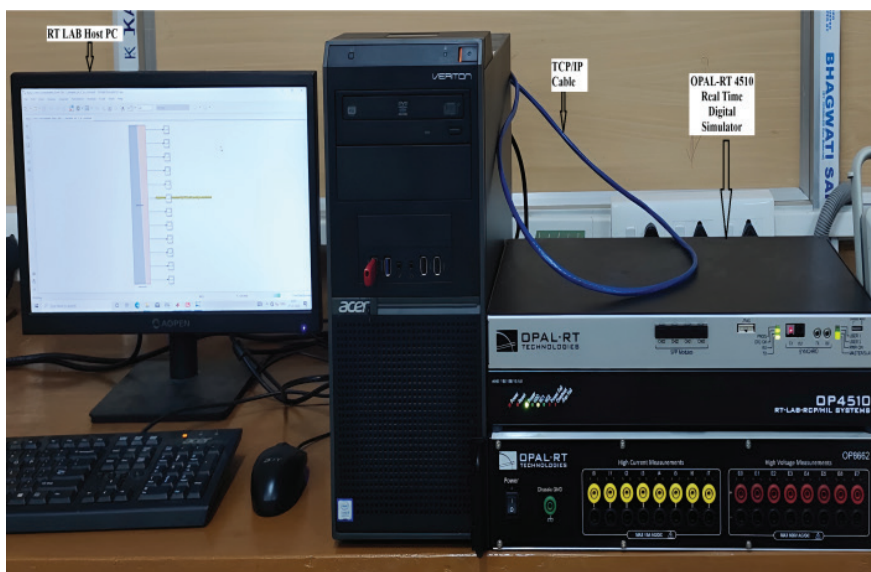
Figure 12. Real-time digital simulation platform installed in the lab.
