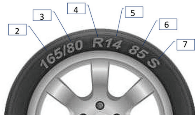
Figure 1. Standardized annotation of tire size.
