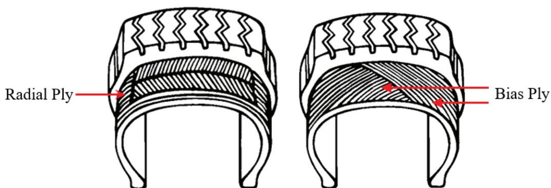
Figure 2. Radial tire configuration with core structural components.
