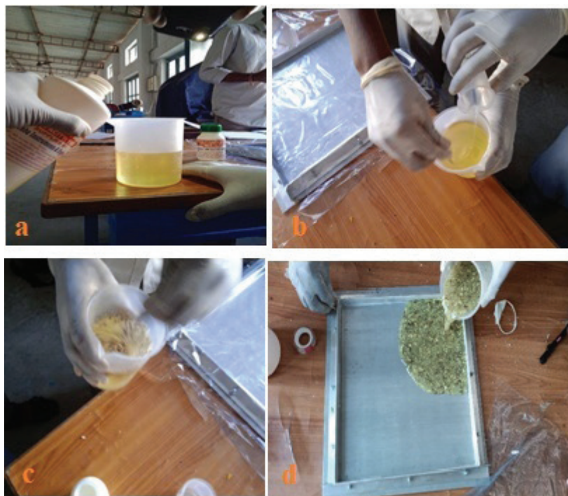
Figure 2. Complete sequential process for fabrication (a) taking of epoxy resin (b) Mixing of hardener mixture with epoxy resin (c) taking fiber sheet and mixing with walnut powder (d) Pouring on fiber sheet uniformly.
