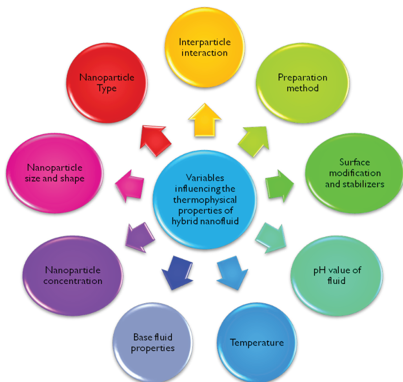
Figure 8. Variables influencing thermophysical properties of hybrid nanofluid.
