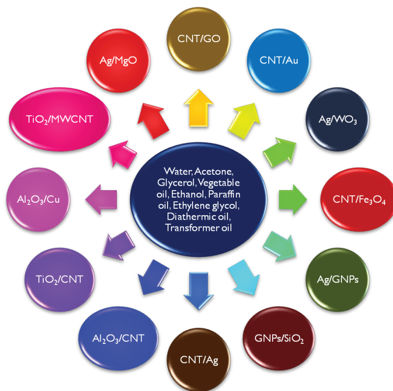
Figure 5. Different base fluid and nanoparticles used in the preparation of hybrid nanofluid.
