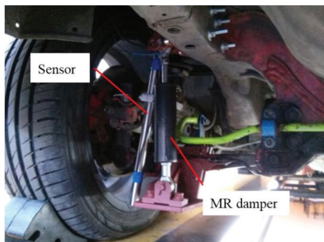
Figure 3. The vehicle is equipped with a control system that utilises a magnetorheological (MR) damper. [From Grzesikiewicz et al. [23], under the terms of the Creative Commons Attribution (CC BY) license.]
