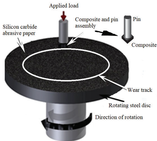
Figure 2. Two-body multi-pass abrasive wear test setup.
