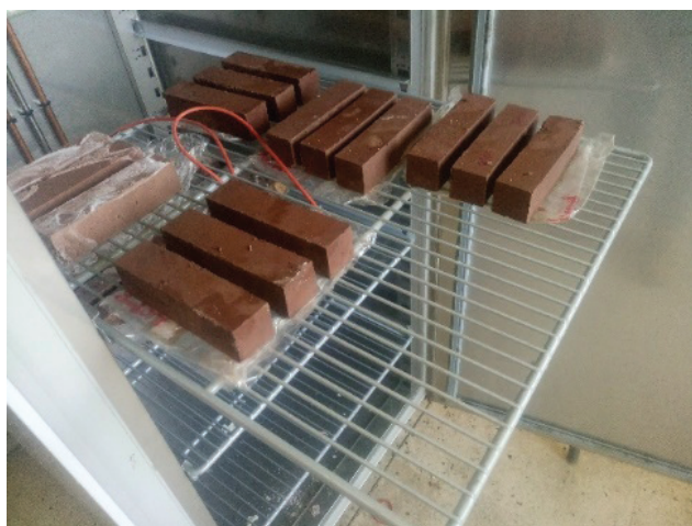
Figure 6. Geopolymer mortar specimens during curing to evaluate their compressive strength.
