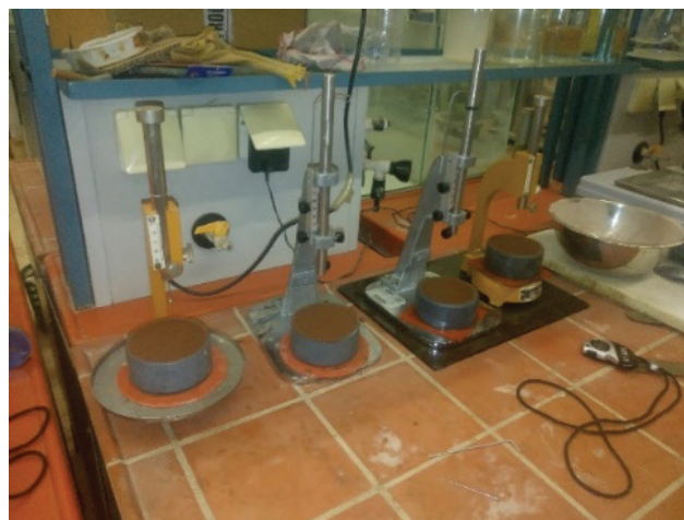
Figure 5. Vicat device while measurement of initial and final setting time.
